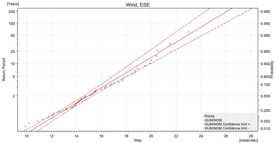
Figure 38: Extreme value analysis for the wind speed ( $W_{sp}$ ) and SE.
