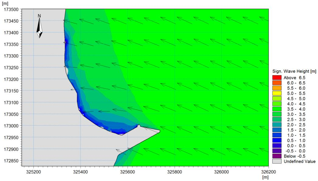
Figure 49: Offshore wave height distribution with waves from the SE. Total computational domain.
