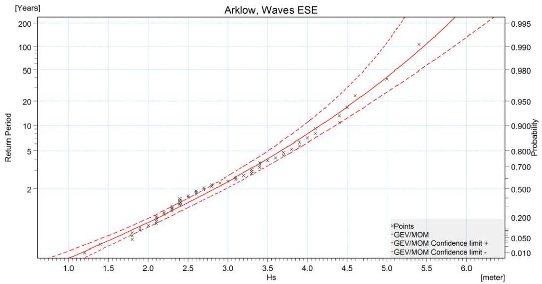
Figure 29: Extreme value analysis for the significant wave height ( $H_s$ ) and SE.
