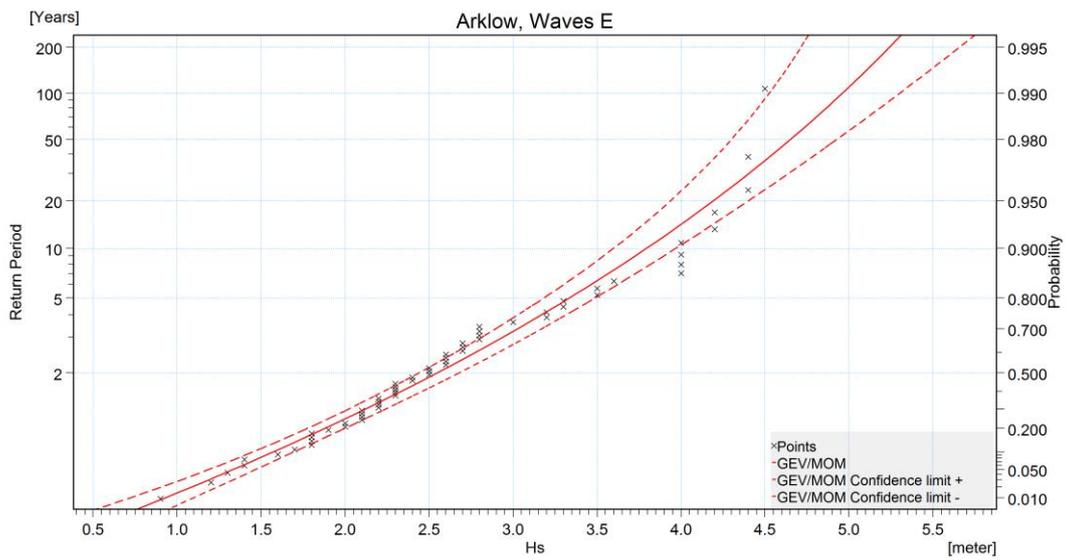
Figure 12: ESE: Extreme value analysis for the significant wave height ( $H_s$ ).
