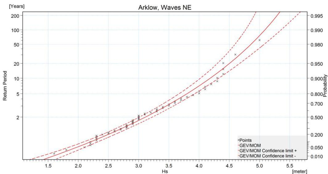
Figure 10: ENE: Extreme value analysis for the significant wave height ( $H_s$ ).
