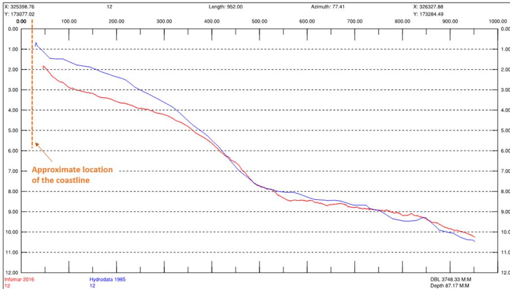
Figure 25: Comparison of 1985 and 2016 bathymetric surveys for profile line no. 15
