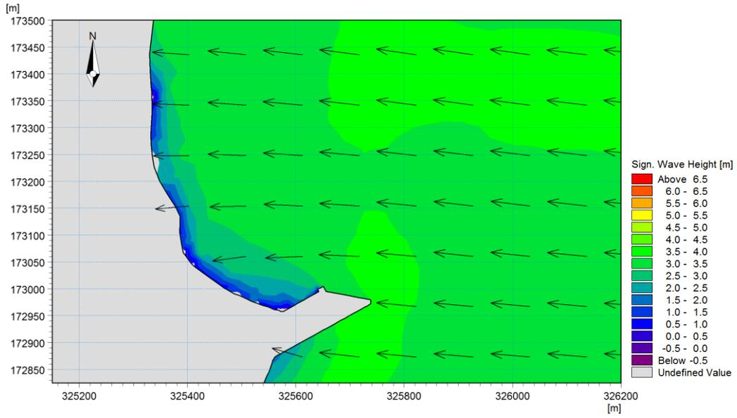
Figure 47: Offshore wave height distribution with waves from the ESE. Total computational domain.
