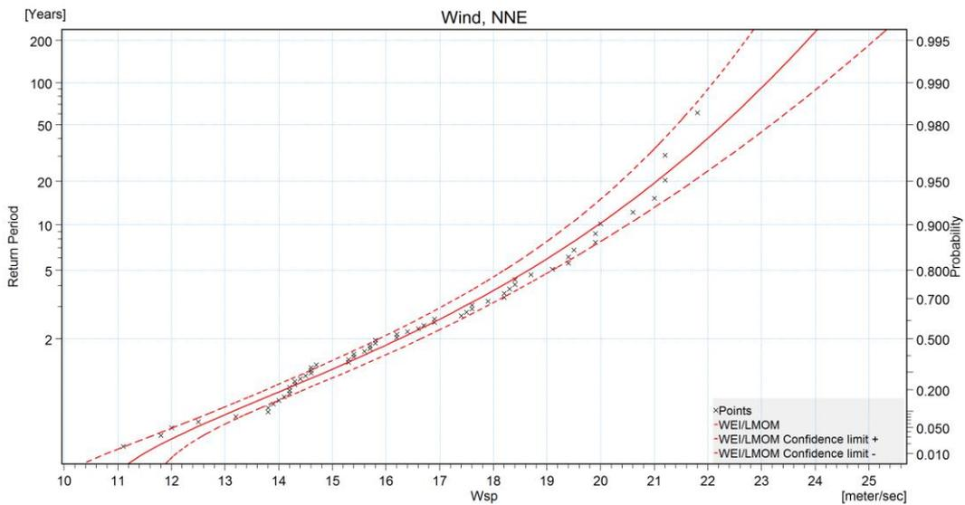
Figure 34: Extreme value analysis for the wind speed ( $W_{sp}$ ) and NE.
