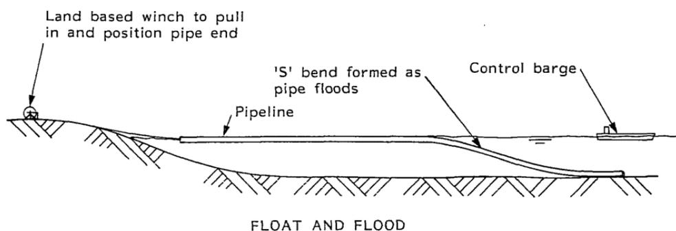
Sections of the outfall pipe would be assembled on land and readied for moving to the water. The pipe and diffuser would be sealed temporarily while full of air, which provides the buoyancy necessary to float.
