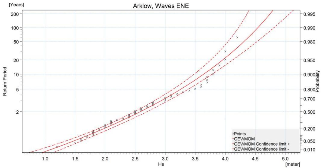
Figure 27: Extreme value analysis for the significant wave height ( $H_s$ ) and E.
