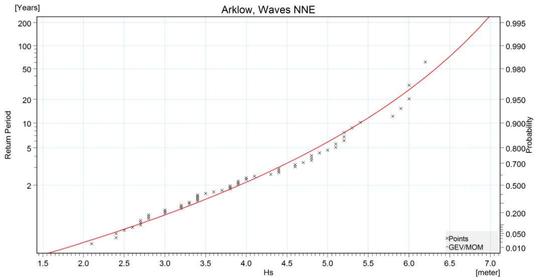
Figure 25: Extreme value analysis for the significant wave height ( $H_s$ ) and NE.
